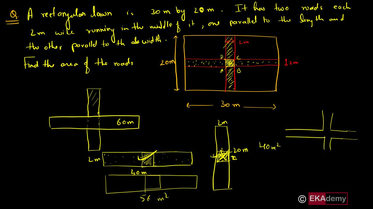
Arredg long wood = 2mx 30m = 60m² Area / Short road = 2m x 20m = 40 m² Area of Square ABCD = # 2m x 2m = 4m<sup>2</sup> Areat & roads = 40 m² +60m² - 4m² = 100 m<sup>2</sup> - 4 m<sup>2</sup> = 96 m<sup>2</sup>
